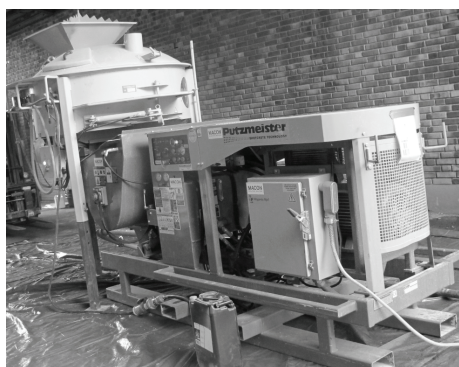
Fig.1 Equipment for pumping and/or shotcreting
