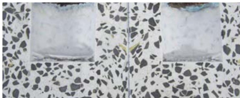
Fig. 8b Alkali resistance of HÖGANÄS PUMP LC 75 AR
