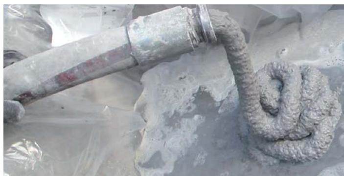
Fig. 3 Pumping of HÖGANÄS PUMP LC 50 AR
