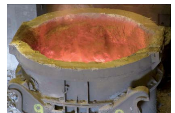
Fig.14. Hot metal ladle lined with HÖGANÄS FLOW LC 70 at SSAB-RaahelFI
